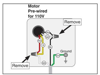
Figure 4. Motor pre-wired for 110V.
